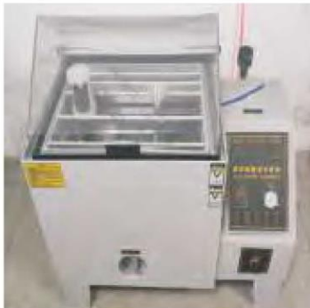
Using Salt spray chamber to analyze the element of stainless steel
